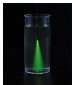
Photograph of a light path from the SoloVPE fibrette dipping into fluorescein solution<sup>1</sup>. The optimal path length is automatically determined by the SoloVPE by searching for a straight line (Abs. vs path length) around 1.0 AU. The vertical position of the fibrette is adjusted accordingly.
