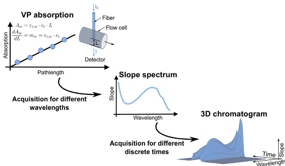
**Fig. 1.** VP spectroscopy in chromatography: Each measurement cycle, variable pathlengths  $L$  are set by actuating the optical fiber of the FlowVPE. After the screening phase for the identification of the optimal measurement pathlengths, UV absorbance spectra at five different pathlengths are acquired. The slope  $m_w$  is calculated for each wavelength giving a slope spectrum. For a whole chromatography run, this results in a 3-dimensional chromatogram in (time, wavelength, slope).
